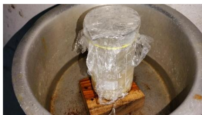
Fig. 27 Heating of swim bladder concentration with 100 ml of water
