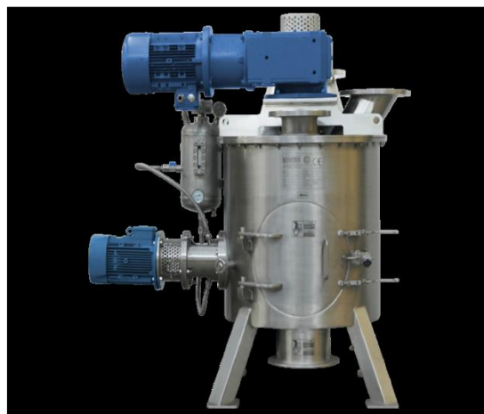
Shifter with sieves of suitable mesh of size.
